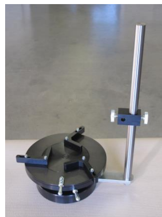
Fig. Jig for measuring bottle perpendicularity in the glass industry
