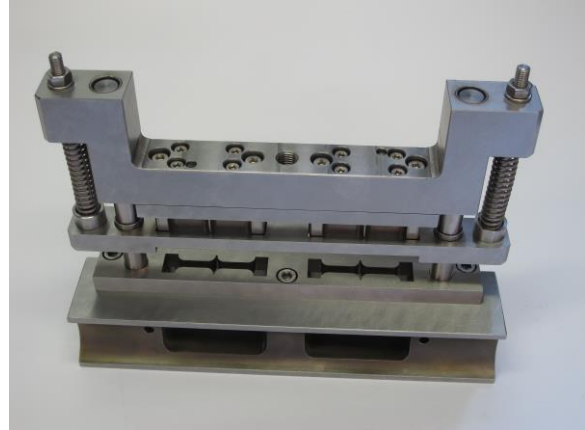
Fig. Cutting unit for packaging machine with waste removal after cutting
