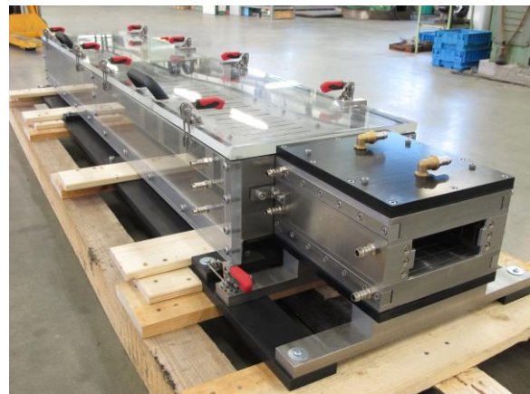
Fig. Calibration and cooling parts of extrusion tool ready for delivery to customer tests
